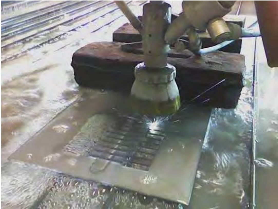
Figure 3-6: Abrasive waterjet cutting of specimens from raw sheet material
