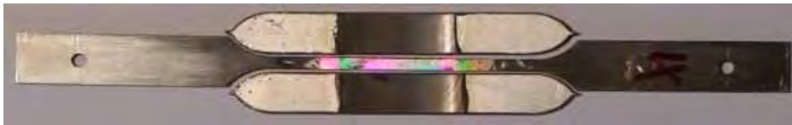
Figure B-7: TAG MS 2 post-test image showing discoloration indicative of residual strain at weld boundaries
