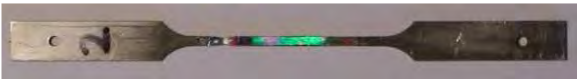
Figure B-1: TAG MS 0 showing visible necking at failure point outside of retreating weld boundary
