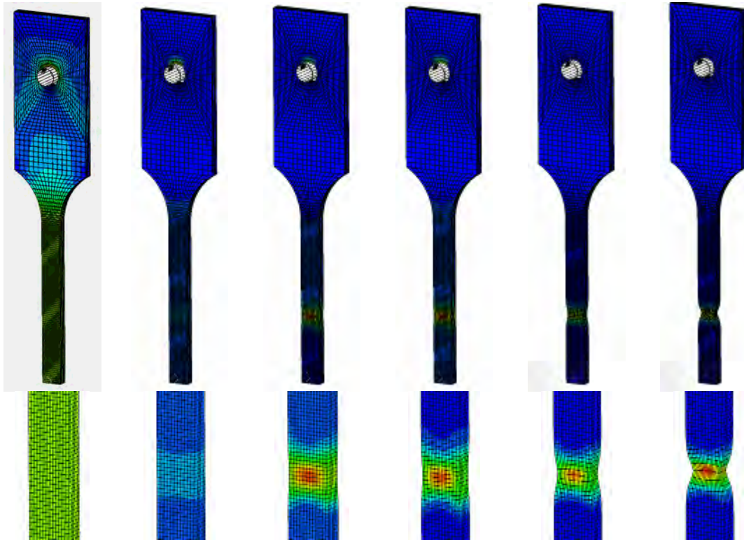
Figure 4-5: Maximum principal strain progression from uniform elastic loading to localized failure
