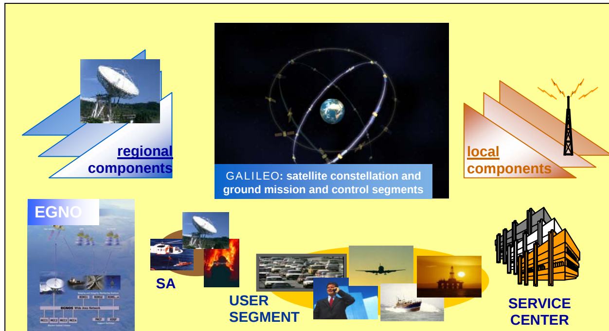
Figure 1. Overall Galileo System overview.
