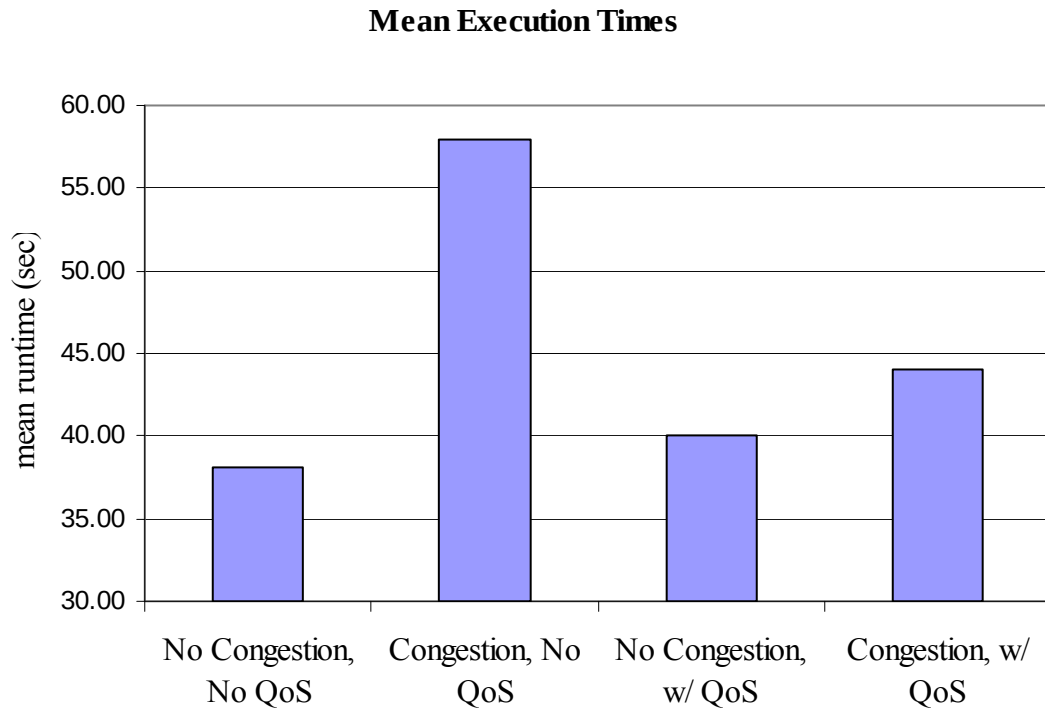
Figure 22. A comparison of RayTracer execution times under different testing conditions. The chart illustrates the time lost due to network congestion, and how the QoS profile prioritized cluster traffic to reduce execution time.
