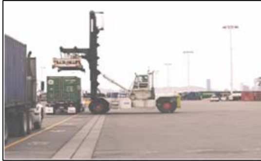
Figure 25. This picture shows a “top picker” releasing a container onto a yard truck or “hustler” at the Port of Oakland in March 2008.
