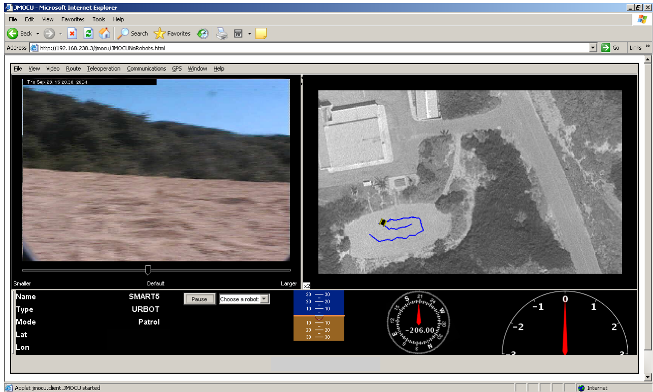
Figure 7. JMOCU is our web-based robot command interface and is a component in SPAWAR's Composible FORCEnet architecture. Multiple robots of many different types can be commanded to perform various actions. Shown here, an URBOT (Urban Robot) is using GPS to navigate along a selected path on the map. On the left is live video from the URBOT. On the right is an aerial image with information about the robot overlaid on top.
