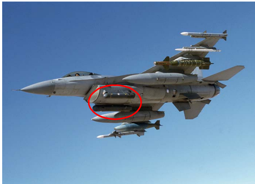
Figure 1. F-16 Aircraft Carrying the LANTIRN System [From (Jane's Avionics, 2006)].
