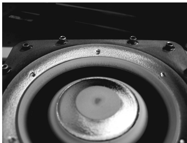
Figure 9. Front surface erosion of a rectangular BHT-600 thruster following extended operation. Note the exposed metal at the thruster center where the protective alumina covering has been eroded.
