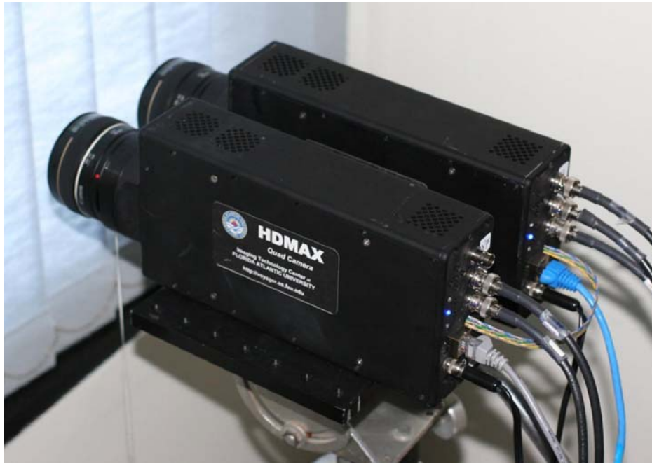
Figure. 3.1. The pair of color HDMAX cameras used for the 3D video imaging system.
