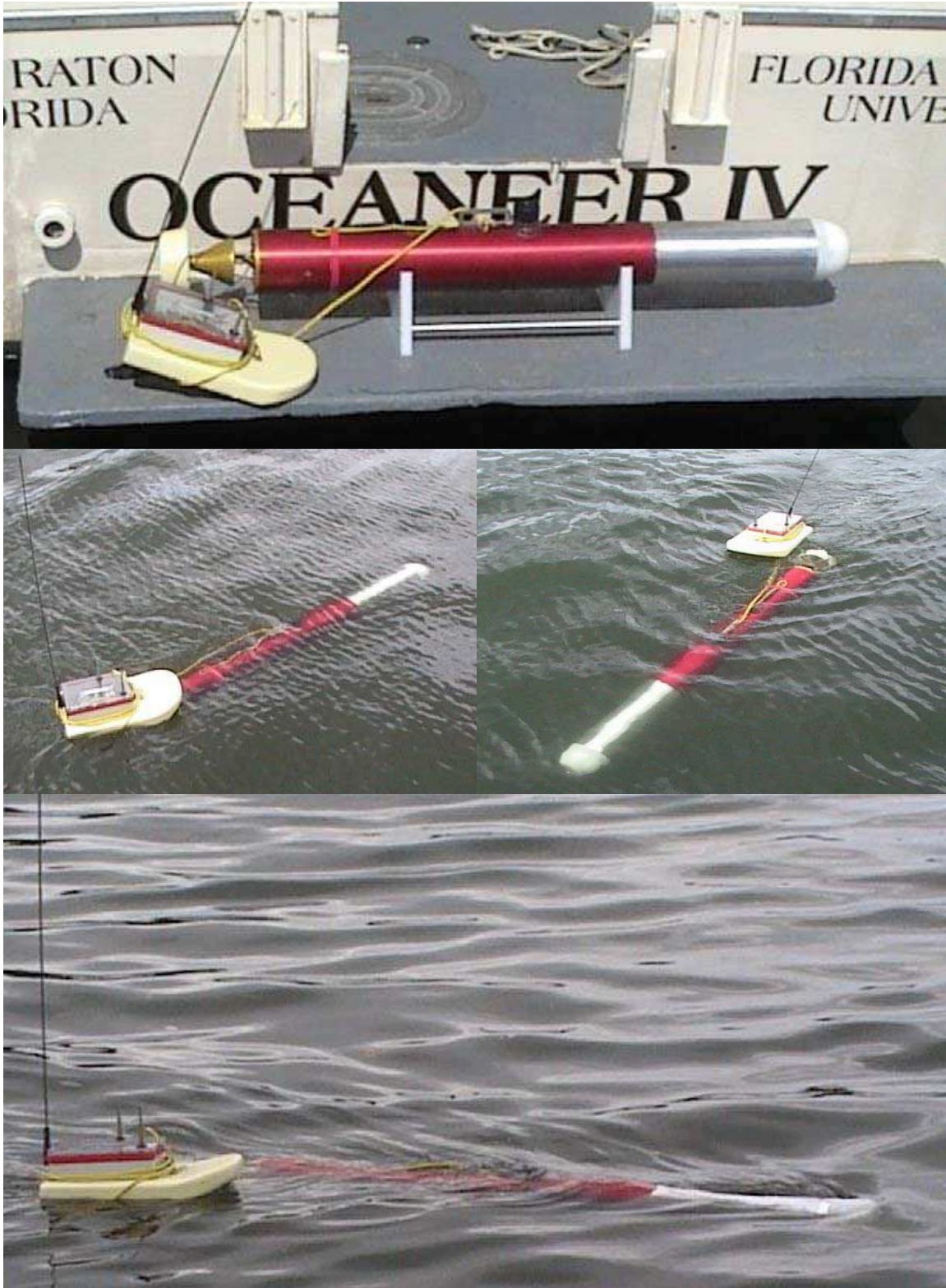
Figure 2.2.16: In-Water Demonstration of the RPUUV with the Chemical Sensor Payload
