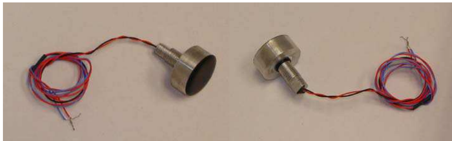
Figure 2.2.3; Obstacle Avoidance Sonar Transducers
