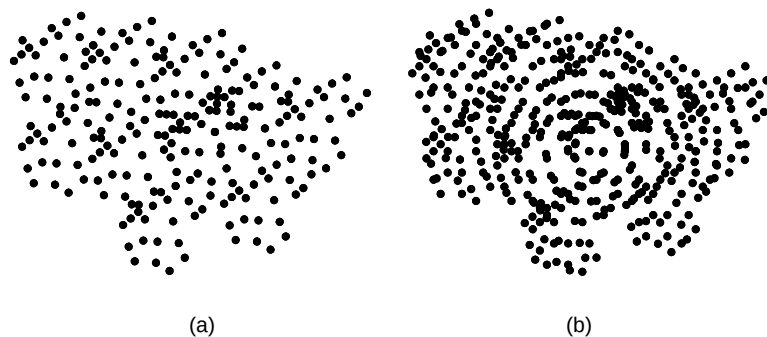
Figure. 3.3. Effect of camera rotation on projected overlay image: (a) with no relative rotation, (b) with several degrees of relative rotation.
