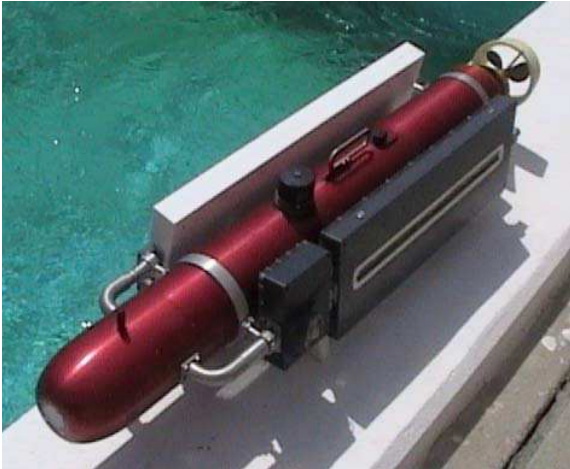
Figure 2.2.21: The RPUUV with the High Resolution Sonar Payload
