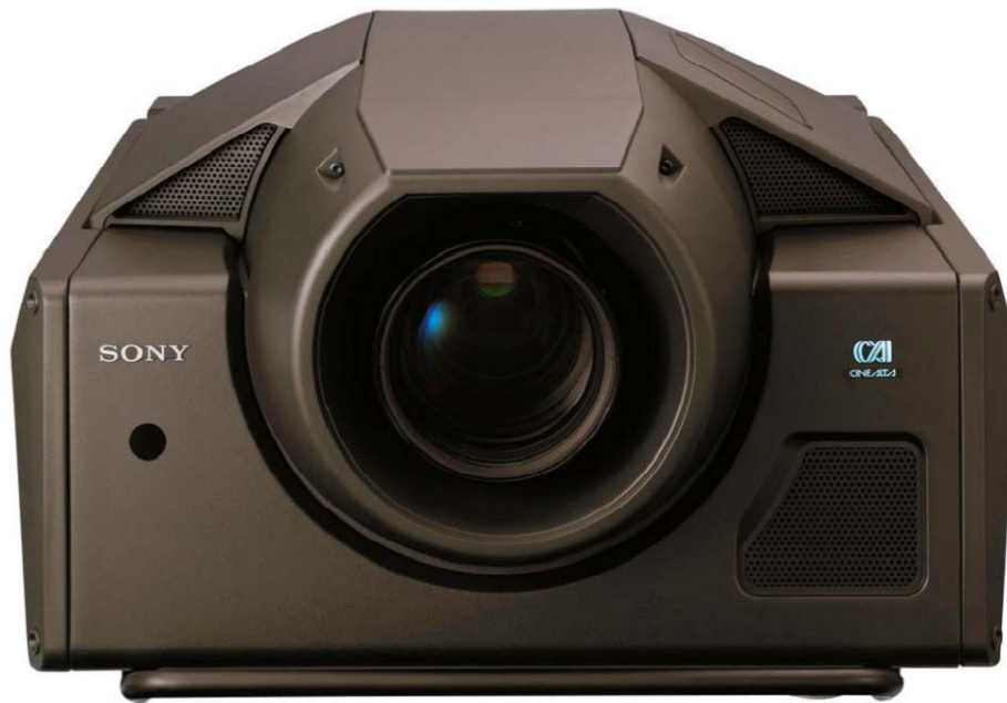
Figure. 3.2. The Sony SRX-R105 digital cinema projector, one of two used for the 3D video display system.
