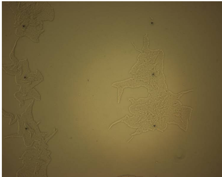
Figure 38. Verified Surface Success. Each successive technique was tested by germinating the spores to see if the technique achieved the criteria of spores in holes while surface is clear. This is a successful demonstration of the discussed rinse and wipe technique.
