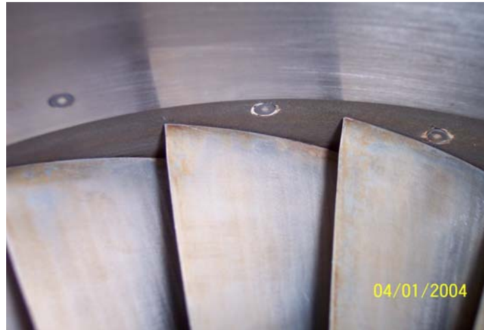
Figure 6. Kulite Probes Mounted Around Compressor Annulus
