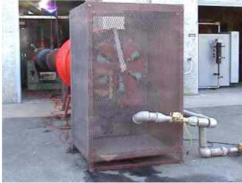
Figure 4. Steam Ingestion System
