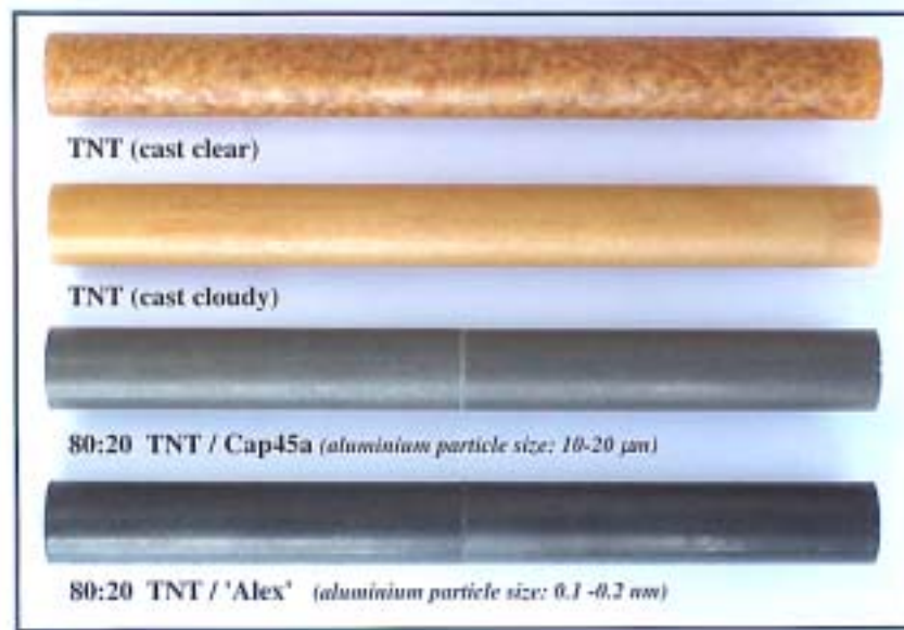
Figure 2. Explosives used in the aquarium tests and the detonation curvature measurements. The samples shown are cylinders 1" (25.4mm) in diameter and 250mm long. Some Tritonal charges were cast in two pieces and then glued together.
