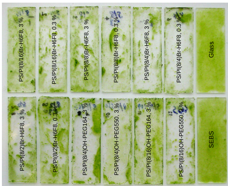
Figure 8. Results of sporeling removal assays on glass microscope slides coated with the SF and PEG containing SABCs of different molecular weights. 3 % and 0.3 % indicate the weight concentrations of the solutions of SABC used for spin-coating.
