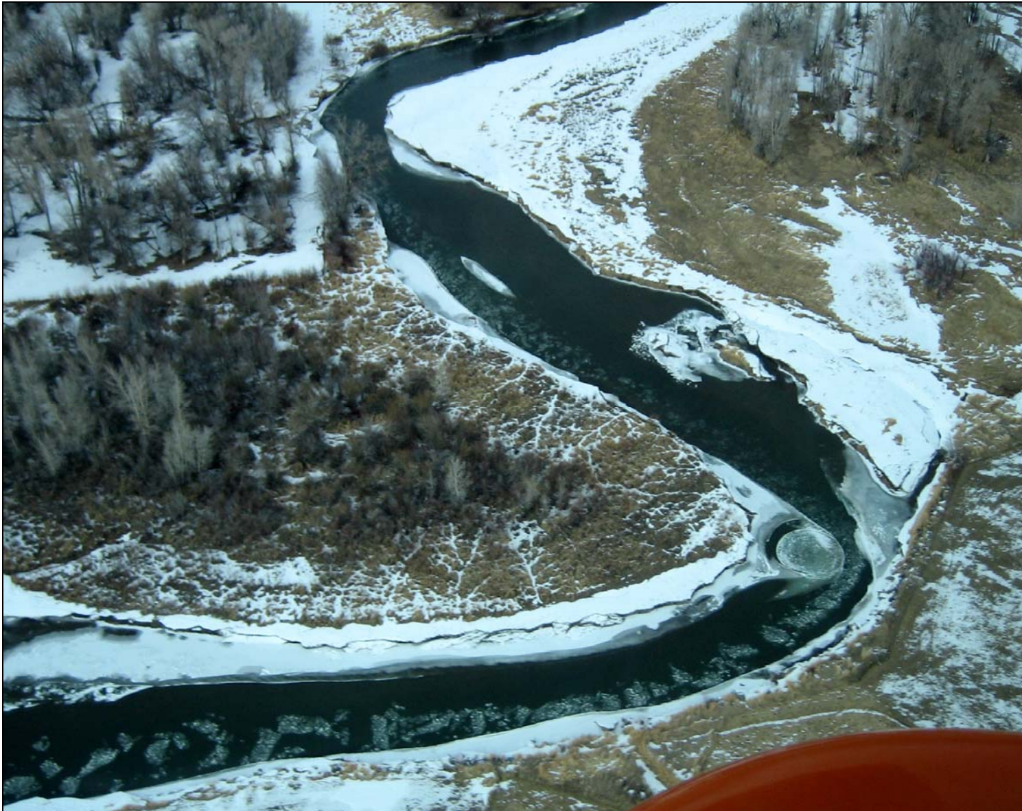
Figure 12. Drifting frazil ice upstream of ice jam on 17 January 2006. Flow direction is right to left.
