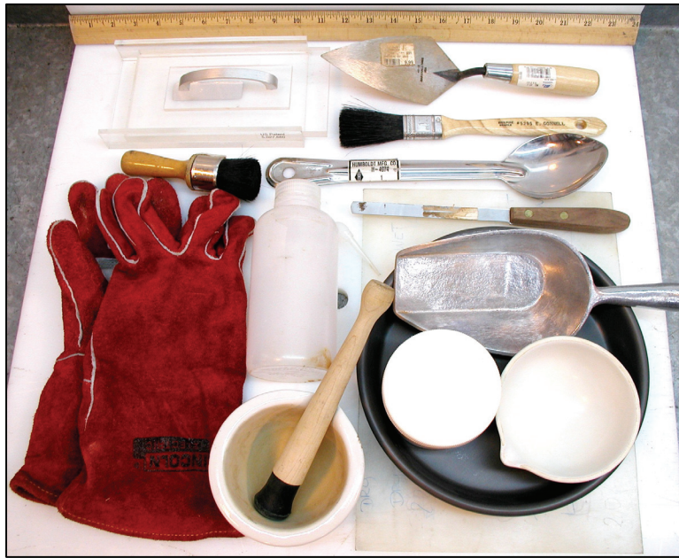
Figure 24. Tools for sampling and processing field soil specimens.
