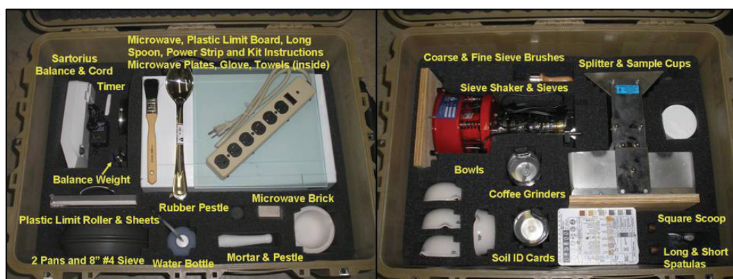
Figure 20. The Rapid Soils Analysis Kit packaged in two Pelican cases.
