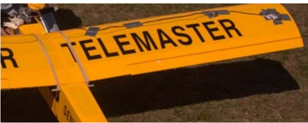
Figure 2. Custom-made dipole antennas mounted on a UAV wing
