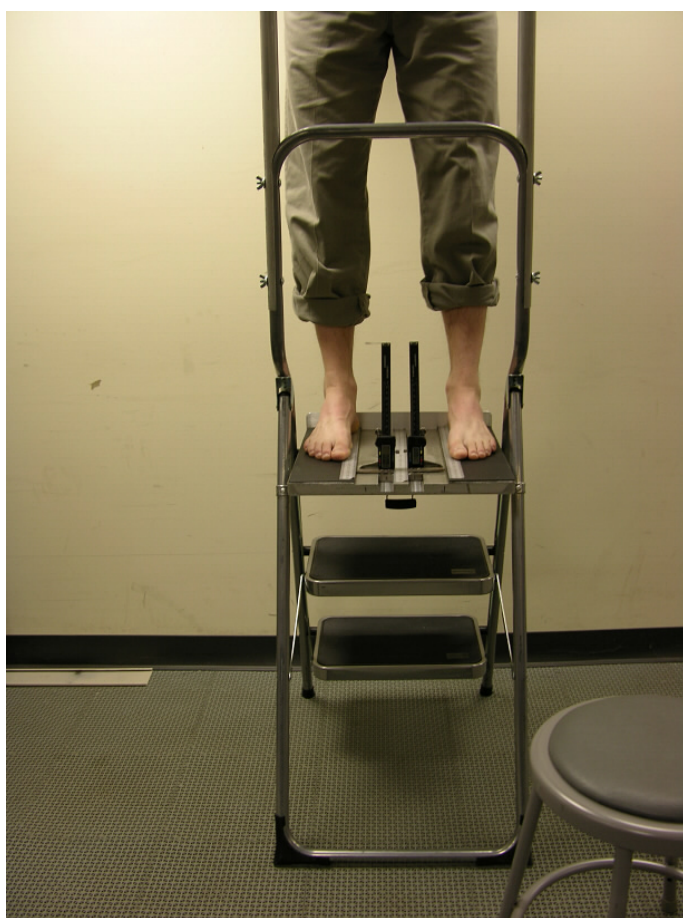
Figure 2. Device Used to Measure Foot Arch Height
