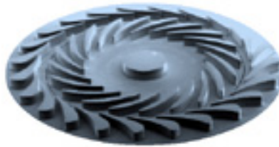
Figure 7: A 4-mm Turbine Wheel Constructed out of Silicon [11]
