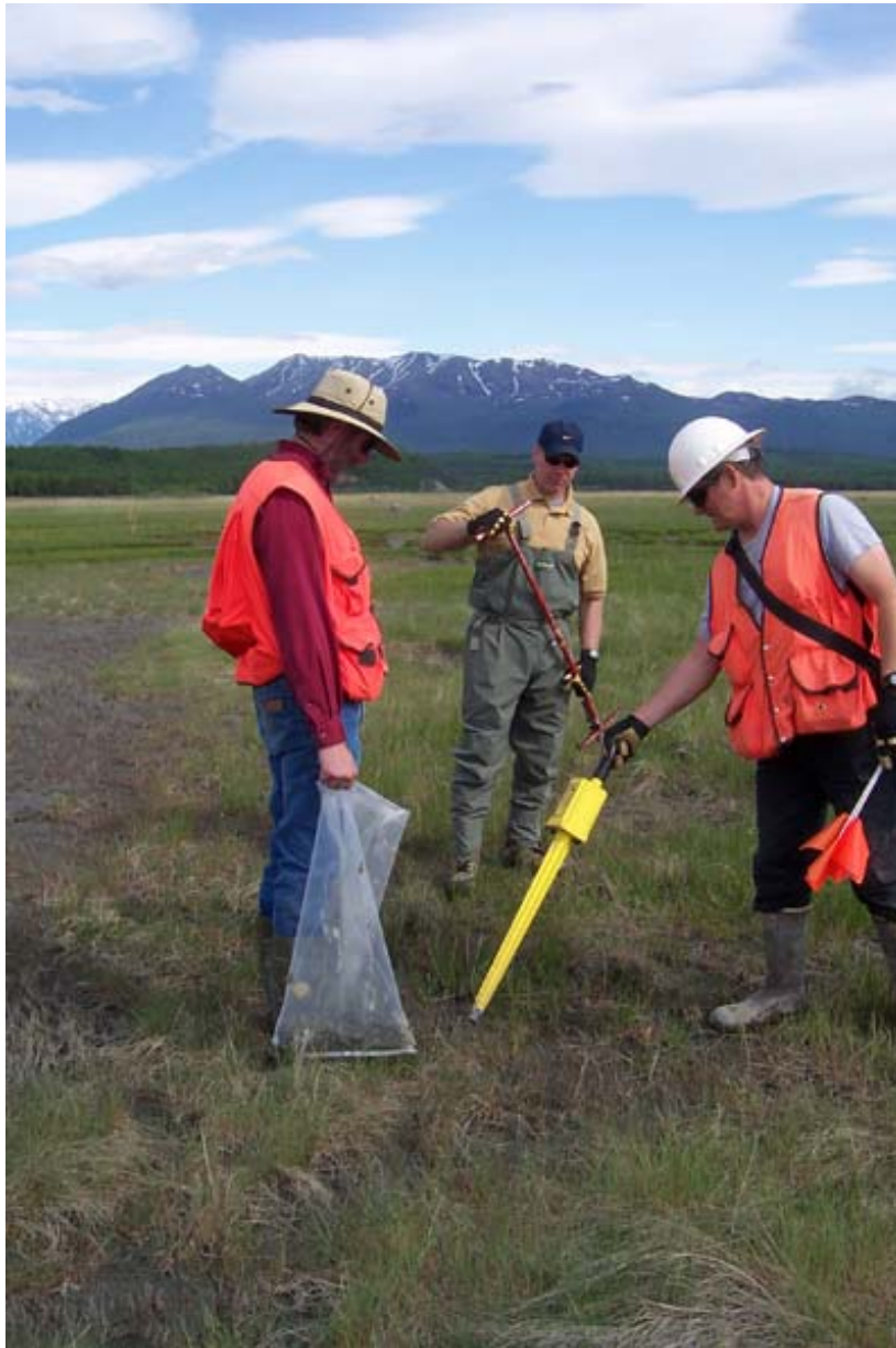
Figure 5. Sampling of 200 m \times 200 m cell. Each point was cleared with a metal detector for potential UXO prior to taking a core.
