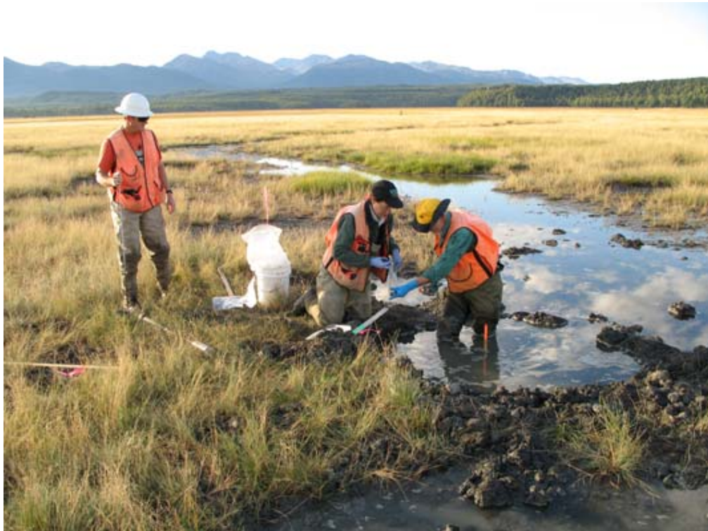
b. Collection of subsurface samples from the same crater after a flooding tide.
