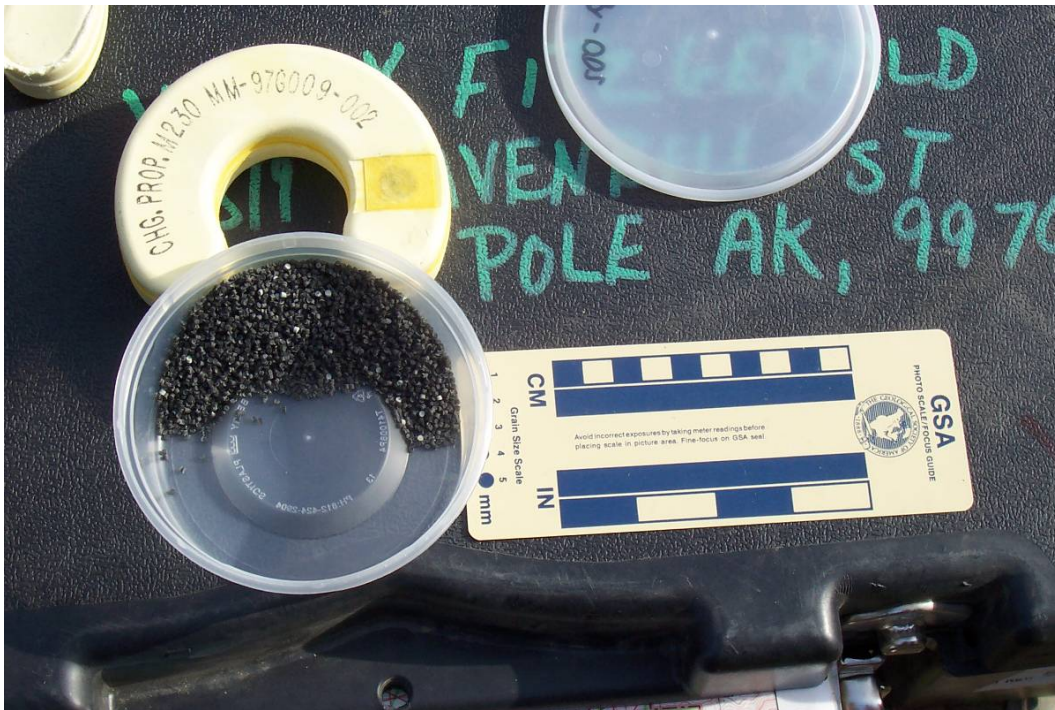
c. M230 propellant charges (containing M45 propellant) for 120-mm HE mortar cartridge.
