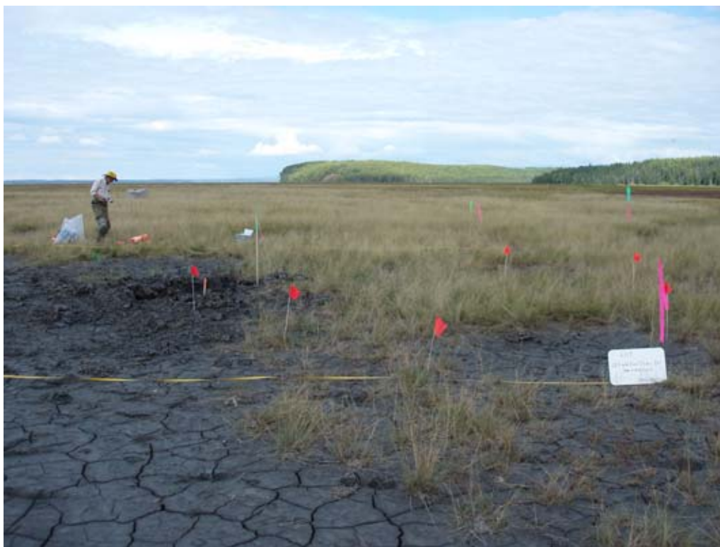
Figure 6. A 10-m \times 10-m area centered on the low-order detonation crater from which multi-increment samples were collected in August 2007 to determine explosives residues. Mean concentrations were 8.8, 4.3, and 1.3 \mu\text{g/g} for RDX, TNT, and HMX.
