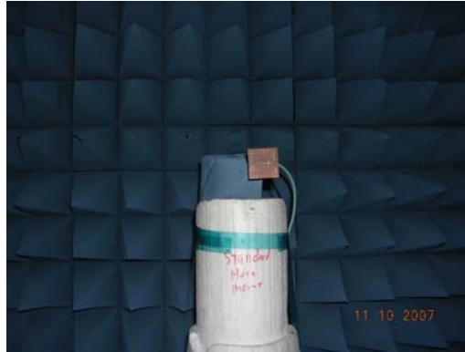
Figure 17. Dipole Antenna/HIGP Measurement in the Anechoic Chamber.
