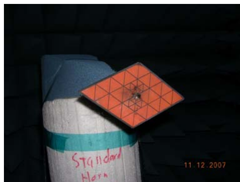
Figure 26. Triangular-patch HIGP with 16 mm-Bow-tie Antenna Measurement
