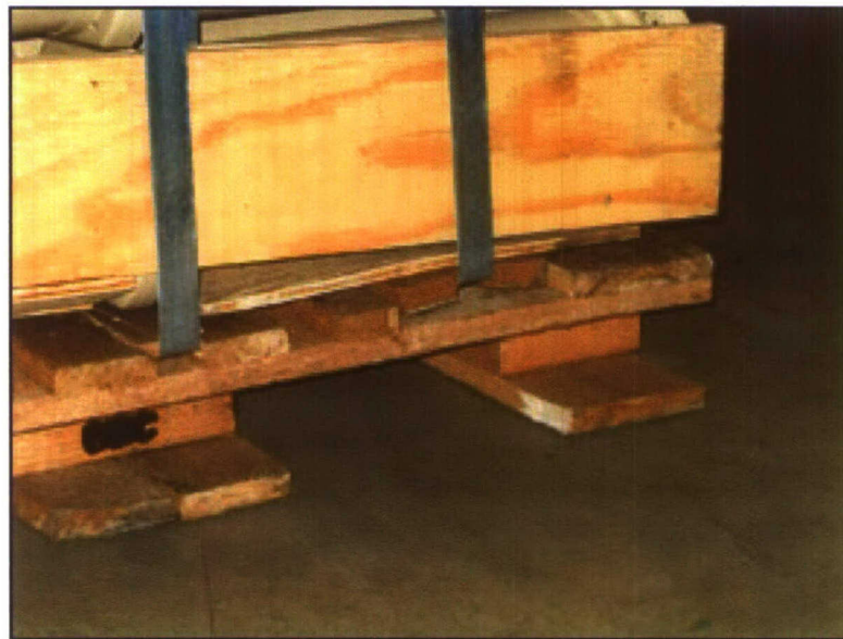
Photo 4. Damage to Wood Pallet
