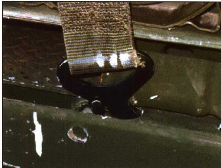
Photo 25. Minor Strap Wear from Container Wall Contact
