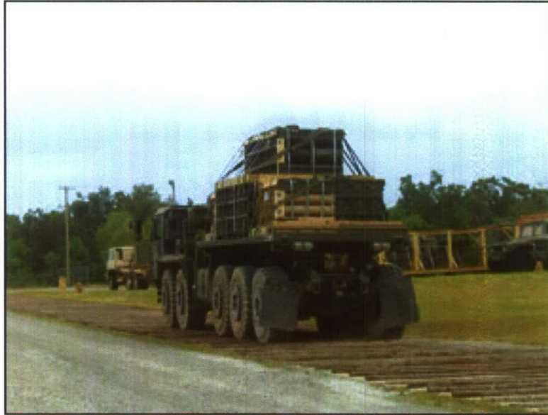
Photo 23. Washboard Course Testing of the Excalibur SCL on the PLS Vehicle
