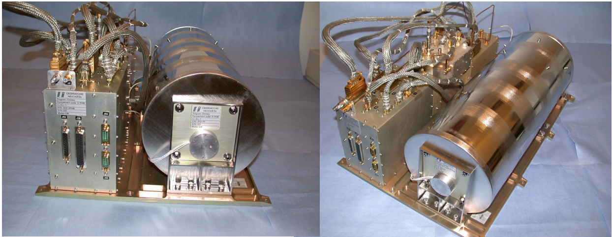
Figure 7. Integrated EM, MLI removed from PP.
