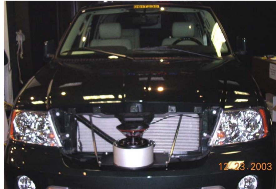
Sensors mounted in grill of Lincoln Navigator
