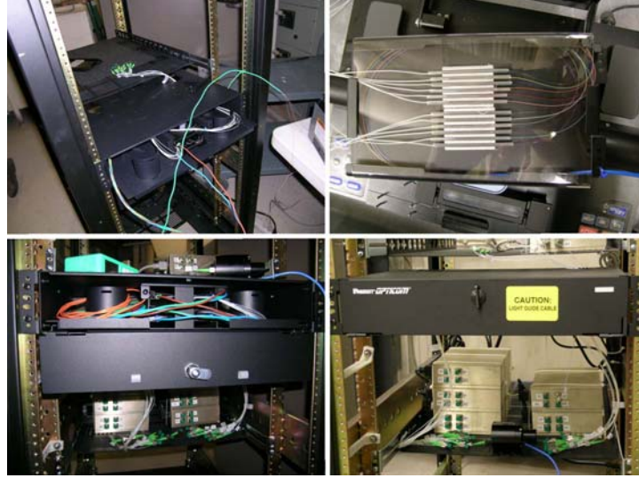
Figure 4. Clockwise from upper left: 1) Initial fiber fan out showing one of the 12-fiber bundles (green) with all of the bare fiber exposed. Also shown are the FC/APC terminations. 2) A splice tray holding 12 splices from bare fiber to the FC/APC termination. 3) The inside of the fan-out enclosure. 4) The final receiver mounting showing the fan-out enclosure, the FC/APC terminations and the receiver modules. Though not shown here, the terminations connect to the inputs on the receiver modules.
