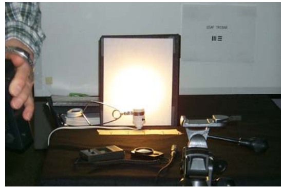
Fig. 3: Position of source relative to target in camera FOV
