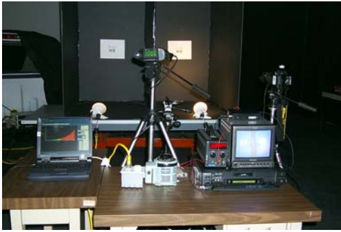
Fig.4: Setup used to measure target luminance
