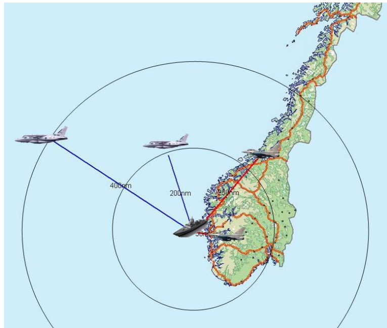
Figure 3.2 Minimum detection ranges of the incoming small airplane threat, assuming that F/A is located either on a regular base or at a forward operating location
