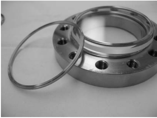
Figure 6. Picture of a sapphire window with knife edge gaskets resting on a vacuum flange. These parts are those shown in Fig. 5 with the exception of the window cap. There is a third copper gasket leaning against the whole assembly.
