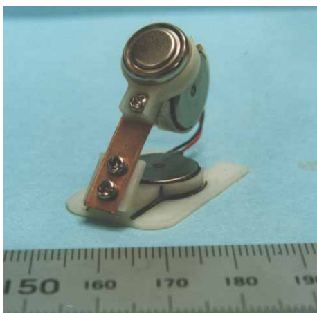
Fig.2 Original tiny hopping robot with resonated cantilever mechanism
