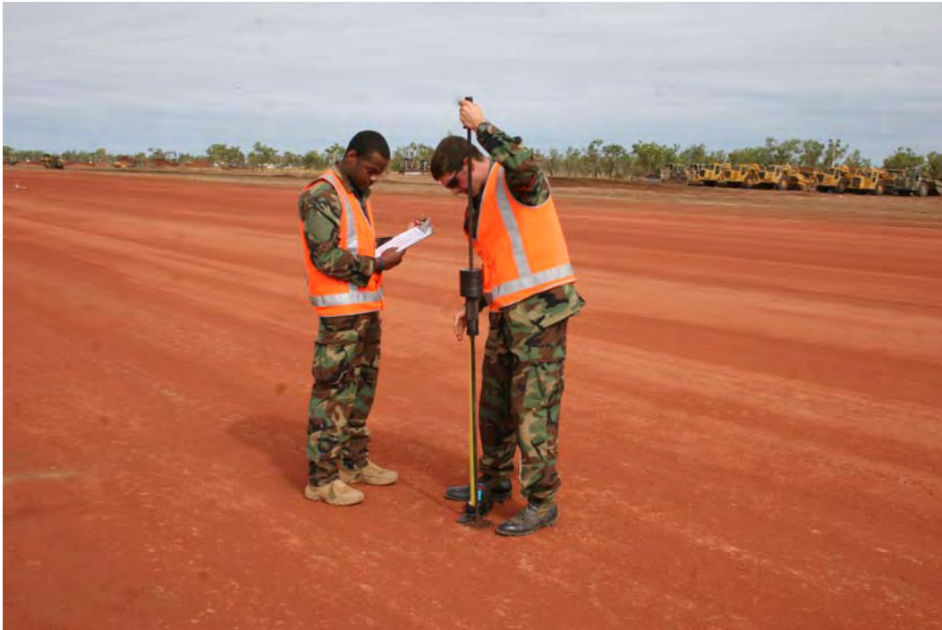
Figure 71. U.S. Air Force conducting DCP tests on runway prior to C-130 arrival.
