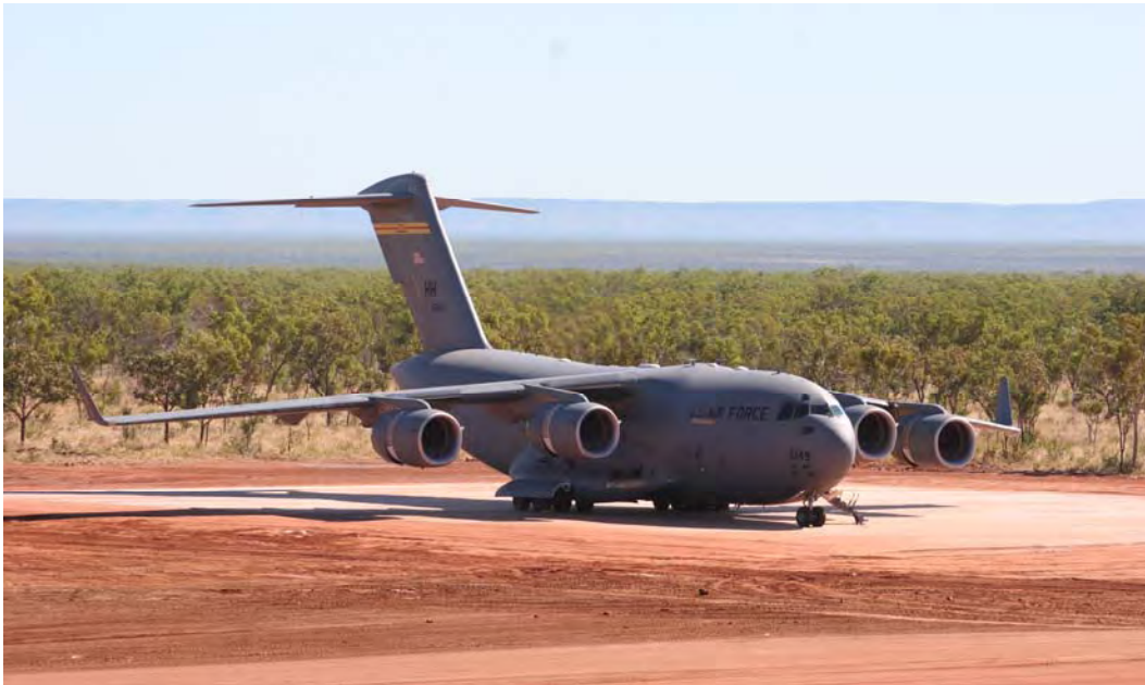
Figure 84. C-17 operating on Apron Alpha less than 24 hr after completion of the stabilization.
