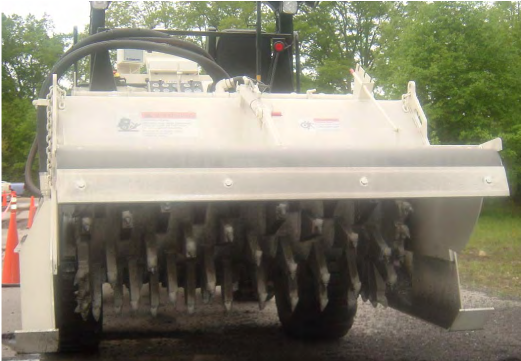
Figure 30. Carbide teeth of the CMI/Terex RS-325B Roto-Mixer (pulvermixer).
