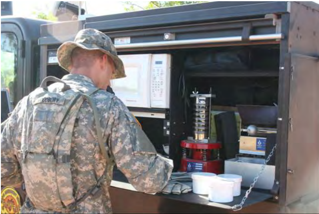
Figure 47. U.S. Army soldier performing a soils analysis on the RAVEN using the RSK.
