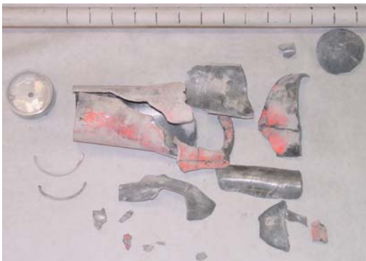
Figure 2. Photograph of the recovered CRH=0.5 projectile pieces from the 529-m/s experiment.
