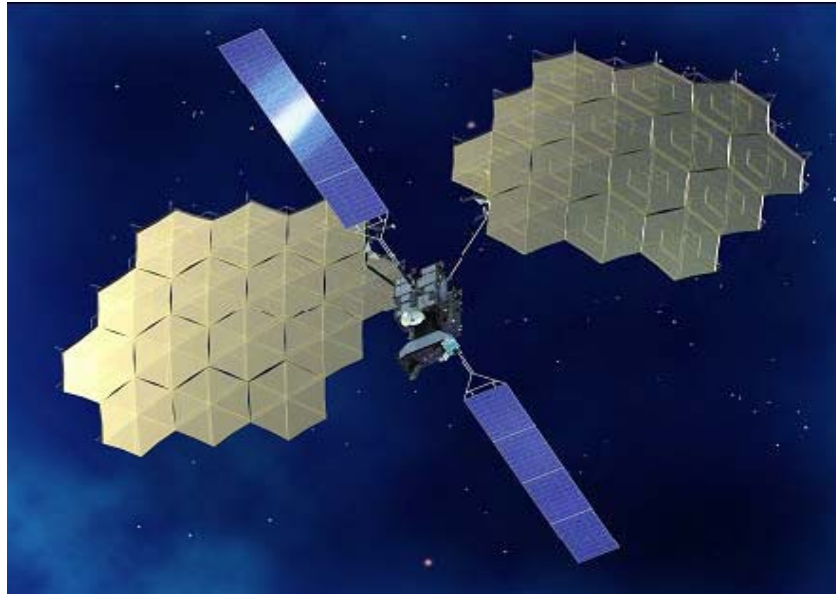
Figure 1. Image of ETS-VIII satellite. The ETS-VIII has two large-scale deployable reflector antennas for development of mobile communications. One reflector size is about the area of two tennis courts.
