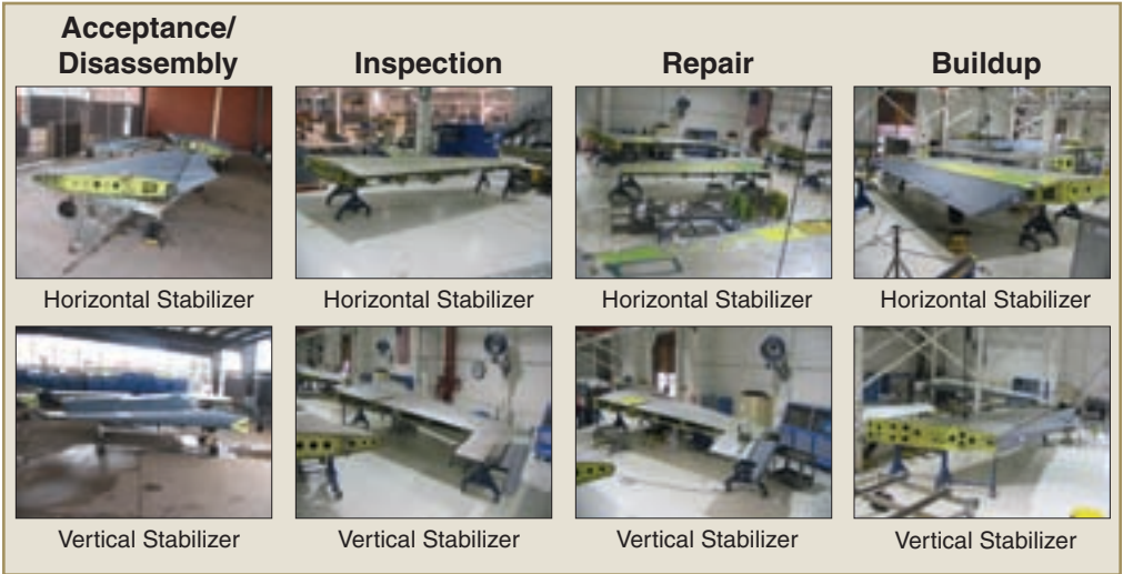
FIGURE 1: HV REPAIR CELL MODEL’S FOUR MILESTONES
