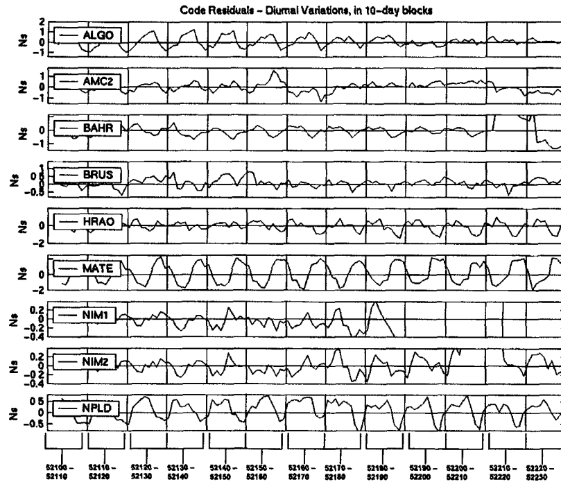
Figure 11. Diurnal signatures in code residuals of continuously filtered carrier-phase GPS solutions, for selected sites, from MJD 52100 through 52220, in 10-day bins. As illustrated in Figures 7 and 8, between each vertical line is a plot representing the average binned value for the 10-day period labeled on the x-axis. Points within the vertical bars represent the average diurnal for the 10-day period: points to the left side are just after UTC 0 hours, the point at the middle of each 10-day block is the average of 10 data taken at UTC 12 hours, and points to the right side approach UTC 24 hours. Formal errors are based upon the fit residuals.
