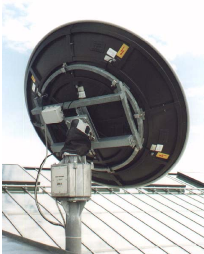
Fig. 6. TWSTFT antenna with support and rotor.
