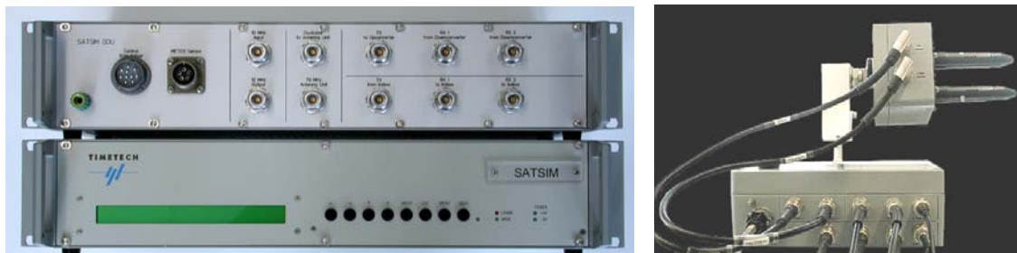
Fig. 7. TWSTFT Satsim Controller and outdoor unit.
