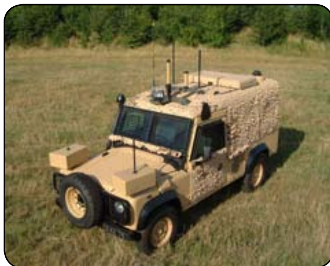
Snatch Landrover fitted with an electronic countermeasures suite as part of an Urgent Operational Requirement
