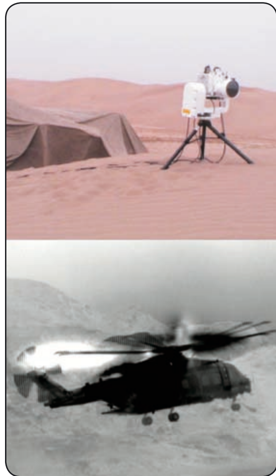
The Thales Quantum Well Infrared Photo-detector (QWIP) camera is an innovative integration of components to produce a cost-effective and affordable Thermal Imaging system; shown during trials in Iraq.
