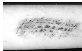
Figure 4. Optical micrograph showing scratches on the surface of a bone specimen stained by Au NPs (dark). The width of the specimen is 5 mm.
