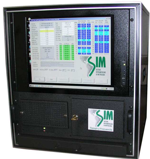
Figure 2. The SIM common-view GPS measurement system.
