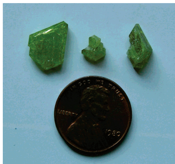
Figure 3. Photograph of Zn_{0.945}Mg_{0.055}O as grown crystals. Pure ZnO crystals were used as seeds.
