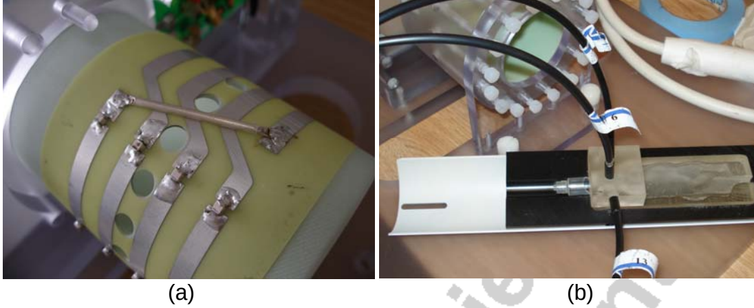
Fig. 5. (a) Photograph of the coil layout showing connected strip conductors and holes to provide access for optical fibers. The custom designed mouse bed accommodates the spectroscopy fiber bundles and fits into the rodent coil for simultaneous MR and optical acquisition (b).
