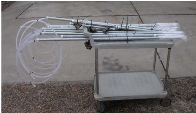
Figure 4-8. Trident probe validation piezometers prior to installation (lower left), installed along transect 3 (upper left), at replicate station T3-3 (upper right), and being sampled (lower right).
