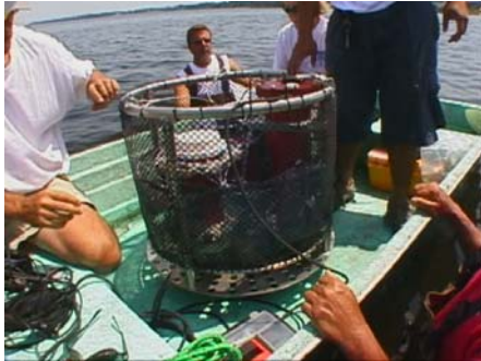
Figure 4-21. The UltraSeep being deployed in Saint Andrews Bay (bottom left and mid), installed on the bottom (bottom right), and viewed from above, including the array of VOC and level logging piezometers at station T4-4 (top).
