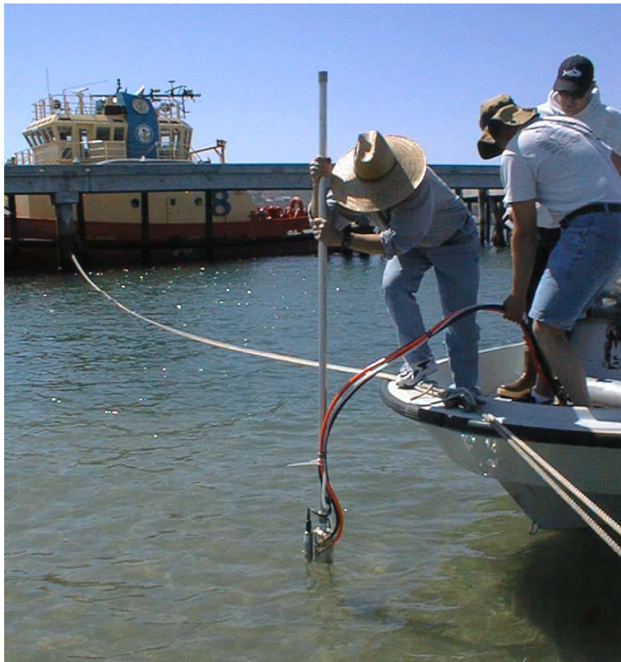
Figure 2-7. Deployment of Trident probe from small boat using push-pole and air hammer.
