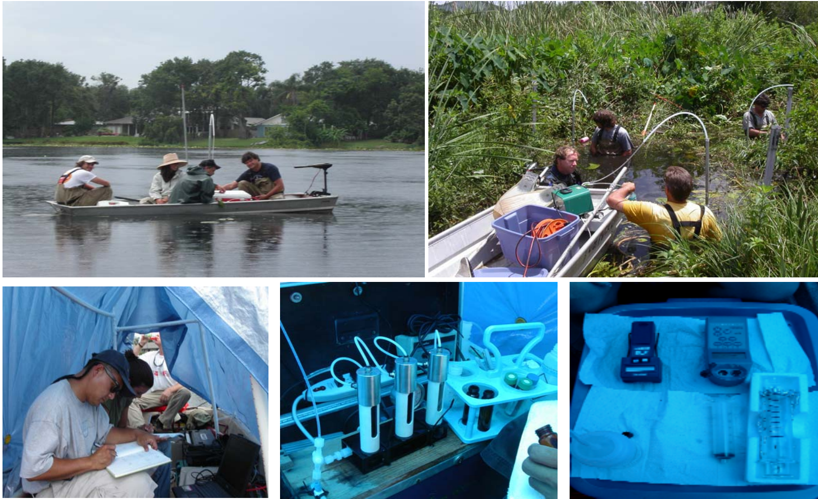
Figure 4-14. Trident probe sampling by small boat (upper left) and wading (upper left), water sampling and data collection (lower left), VOA sampling manifold (lower mid), and water quality analyzers (lower right).
