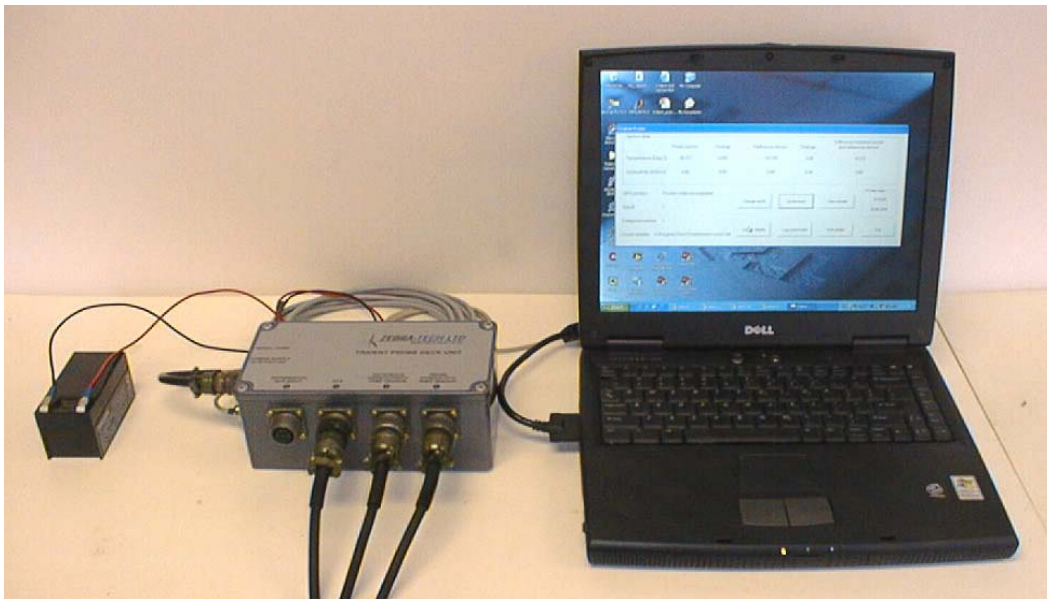
Figure 2-5. Trident probe deck unit interfaced to a laptop. Small gel-cell battery powers Trident probe sensors.
