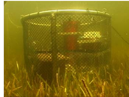
Figure 4-21. The UltraSeep being deployed in Saint Andrews Bay (bottom left and mid), installed on the bottom (bottom right), and viewed from above, including the array of VOC and level logging piezometers at station T4-4 (top).
