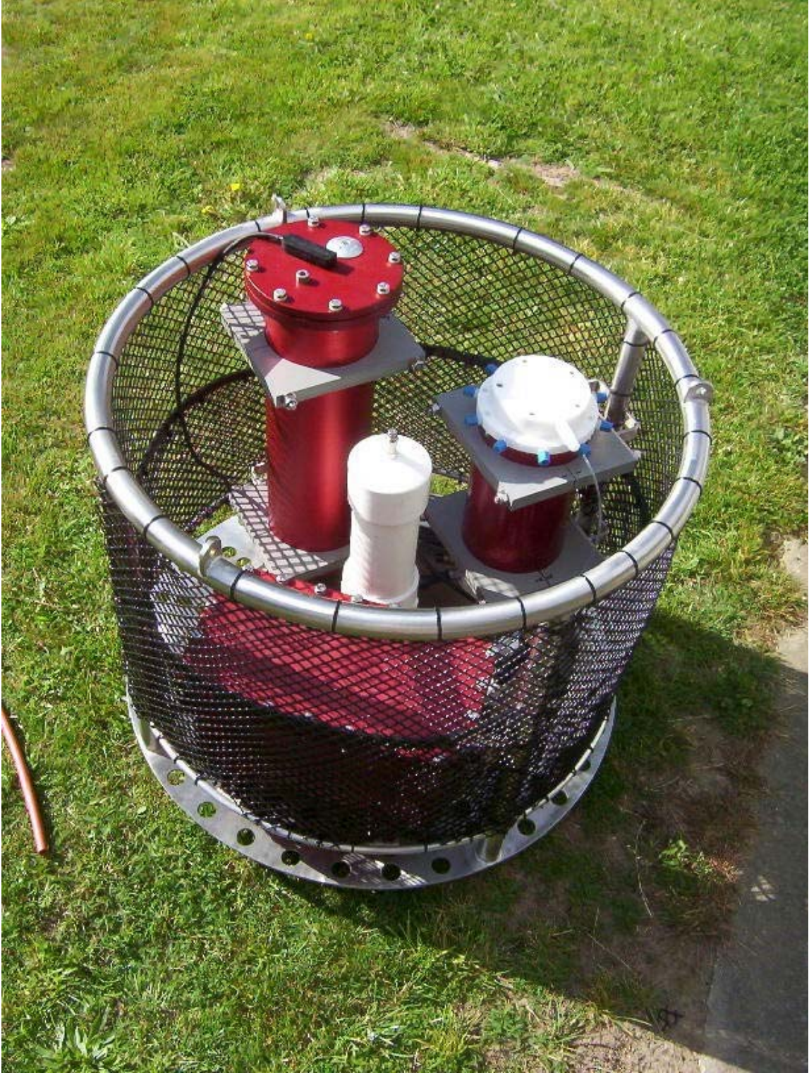
Figure 2-10. Oceanscience Group commercial UltraSeep system.
