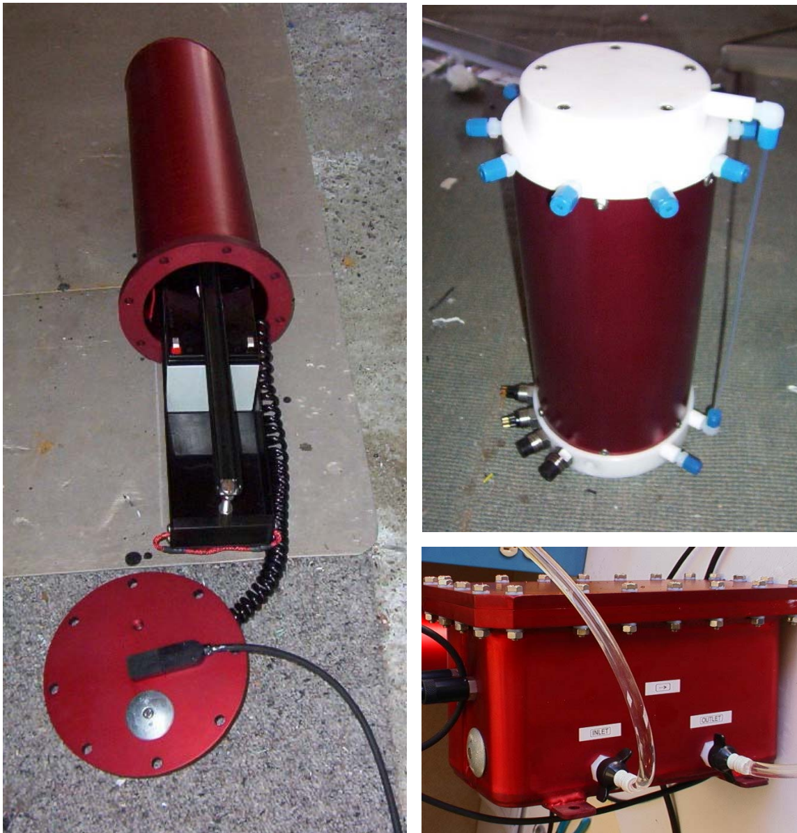
Figure 2-12. Individual UltraSeep components, including battery (left; shown opened), sampling system and control unit (upper right), and flow meter (lower left).
