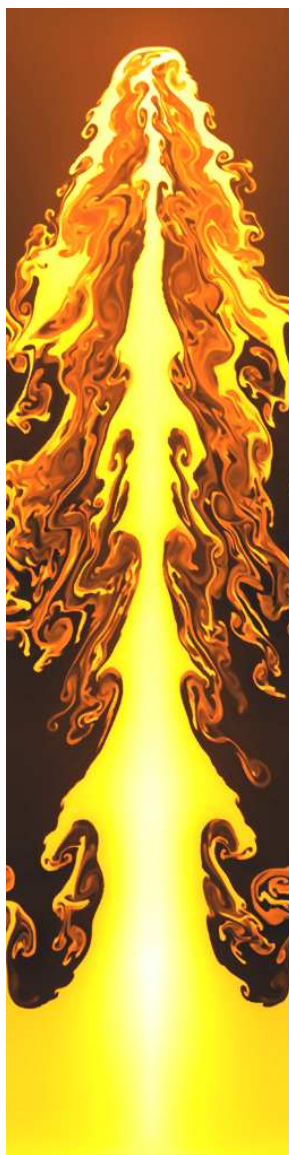
Figure 9. Solution of Rayleigh-Taylor instability at t = 2.5 as computed with the current framework.
