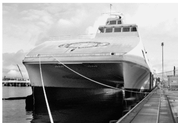
Figure 8: The US Navy experimental ship SEA FIGHTER (FSF1) is 262 feet long, with a beam of 72 feet. Four water jets that are powered by two LM2500 gas-turbine engines or two diesels can drive its 950-ton weight over 50 knots. Source. Department of Defense.
