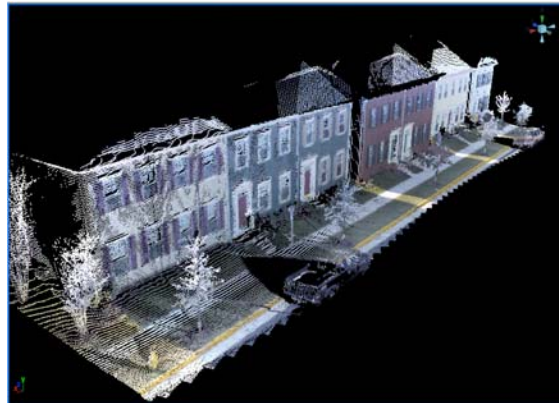
Figure 3: Suburban Washington DC - 2D Rendering of 3D Image Processed Using Leica Cyclone Software
