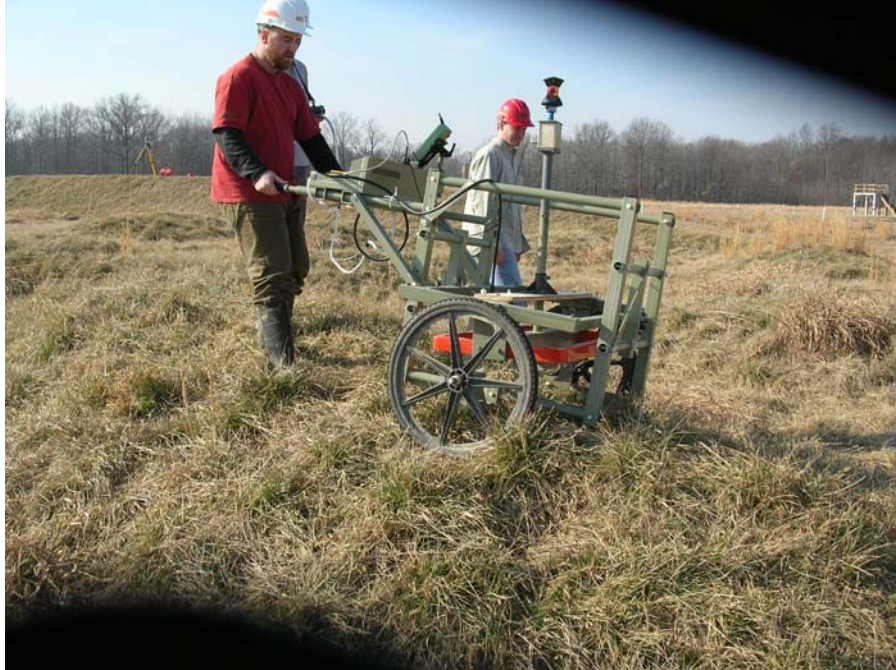
Figure 1. Demonstrator's system, EM61 MKII/pushcart.
