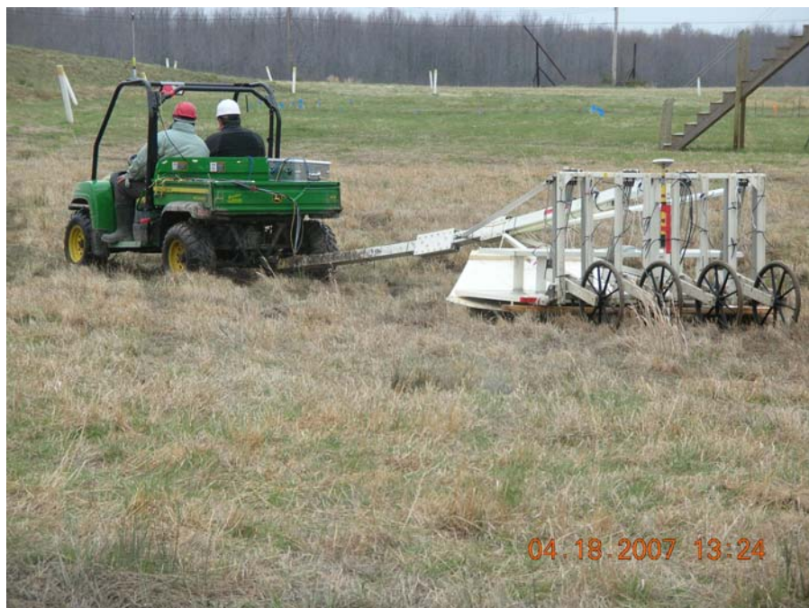
Figure 1. Demonstrator's system, EM AMOS/towed.
