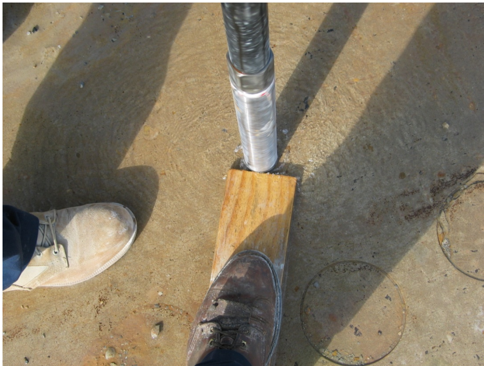
Figure 7. Operators Using Lumber Plank to Keep Drill Plumb while Starting Core
