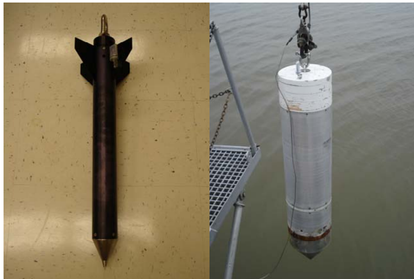
Figure 17. 3 and 9-inch diameter experimental penetrometers
