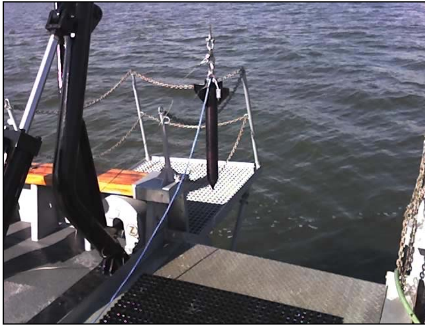
Figure 18. Stern deck view of Oceanography YP, showing U-frame and 3-inch penetrometer
