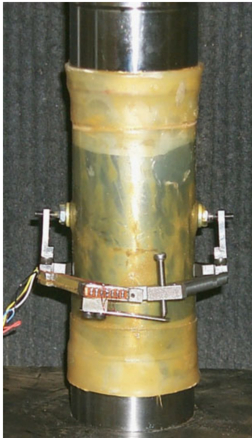
Figure 1. Spring-arm lateral LVDT mounted on test specimen.
