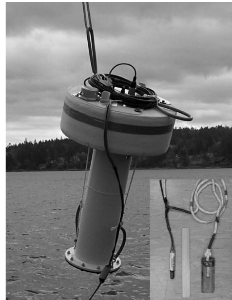
FIG. 1. Photograph of a BURB during deployment from the CCGS Vector, April 2005. Inset at lower right shows the hydrophone, cable, strength member, and lead weight.
