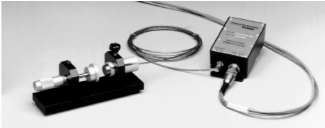
Figure 10. Typical Eddy Current setup for the Kaman Model KD-2300. The sensor itself is mounted in the fixture to the left with cabling leading to an electronics module shown on right.
